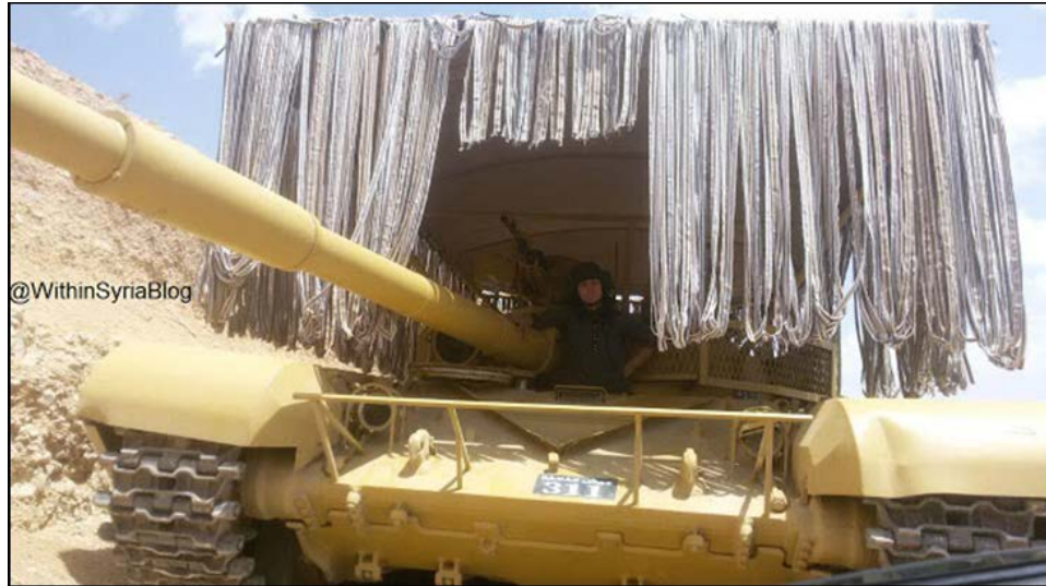
Figure 37. T-72 Ural #311 Tank with Multi-spectral Camouflage. Source: Mitzer and Oliemans (2017c).
